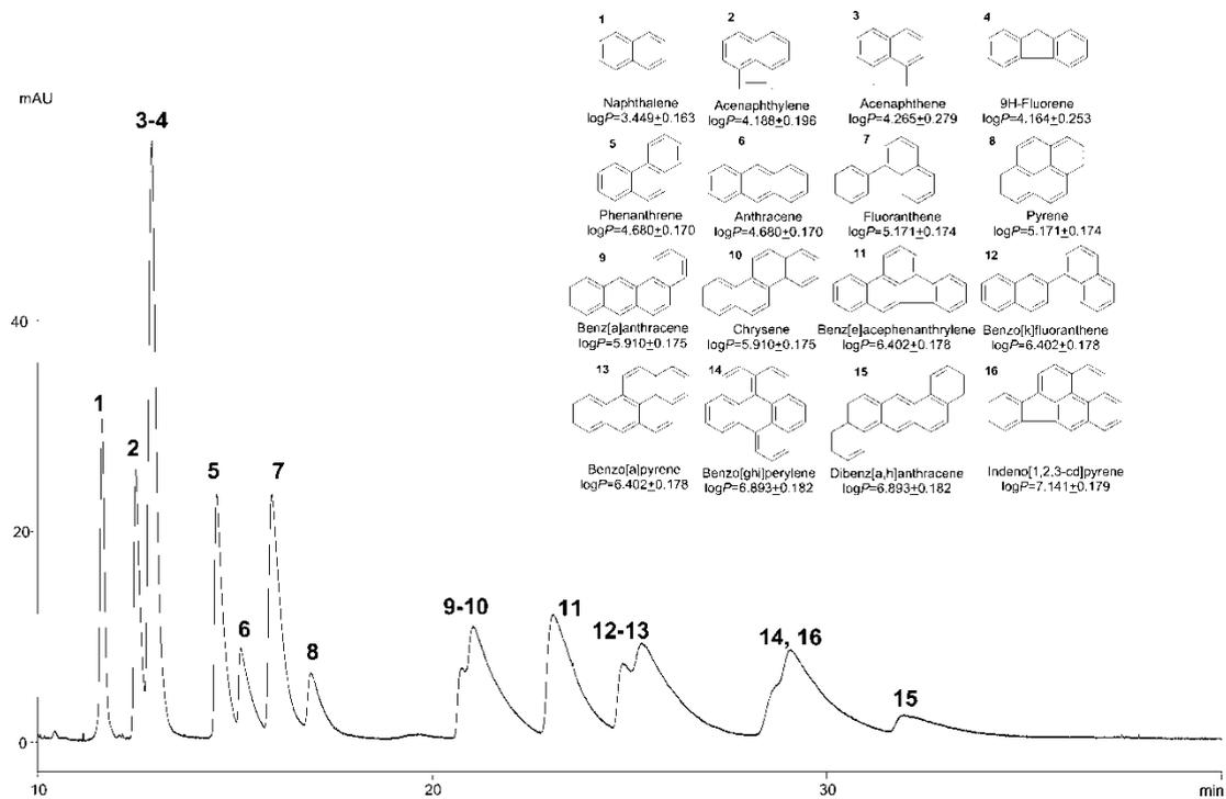
**Figure 2.** Electropherogram of CEC-UV separation of a test mixture of 16 PAHs using the PSG column. The peak identification is listed in the inset. Conditions: 100  $\mu\text{m}$  (I.D.) 30 cm long PSG capillary, mobile phase ACN/H<sub>2</sub>O 50:50 (v/v) containing 5 mM NH<sub>4</sub>OAc at pH 8.0, 10 kV, 25°C, UV detection at 214 nm.
