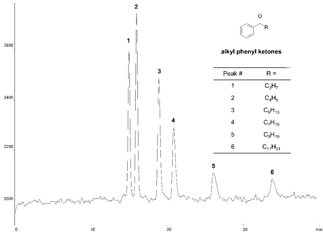
**Figure 5.** Electropherogram of CEC-APPI-MS separation of alkyl phenyl ketones using the PSG column. The conditions are same as Figure 4 or described in experimental section.
