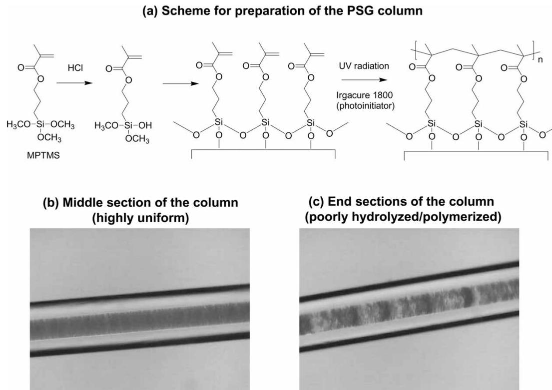
**Figure 1.** (a) Scheme for preparation of the PSG column. Microscopic images showing middle (b) and end (c) sections of the PSG column.
