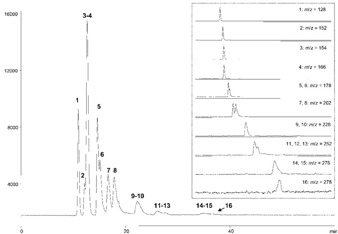
**Figure 4.** Electropherogram of CEC-APPI-MS separation of PAHs using the PSG column. Conditions: 100  $\mu\text{m}$  (I.D.) 65 cm long PSG capillary, mobile phase ACN/H<sub>2</sub>O 50:50 (v/v) containing 5 mM NH<sub>4</sub>OAc at pH 8.0, 10 kV, 25°C. For the other conditions see experimental section.
