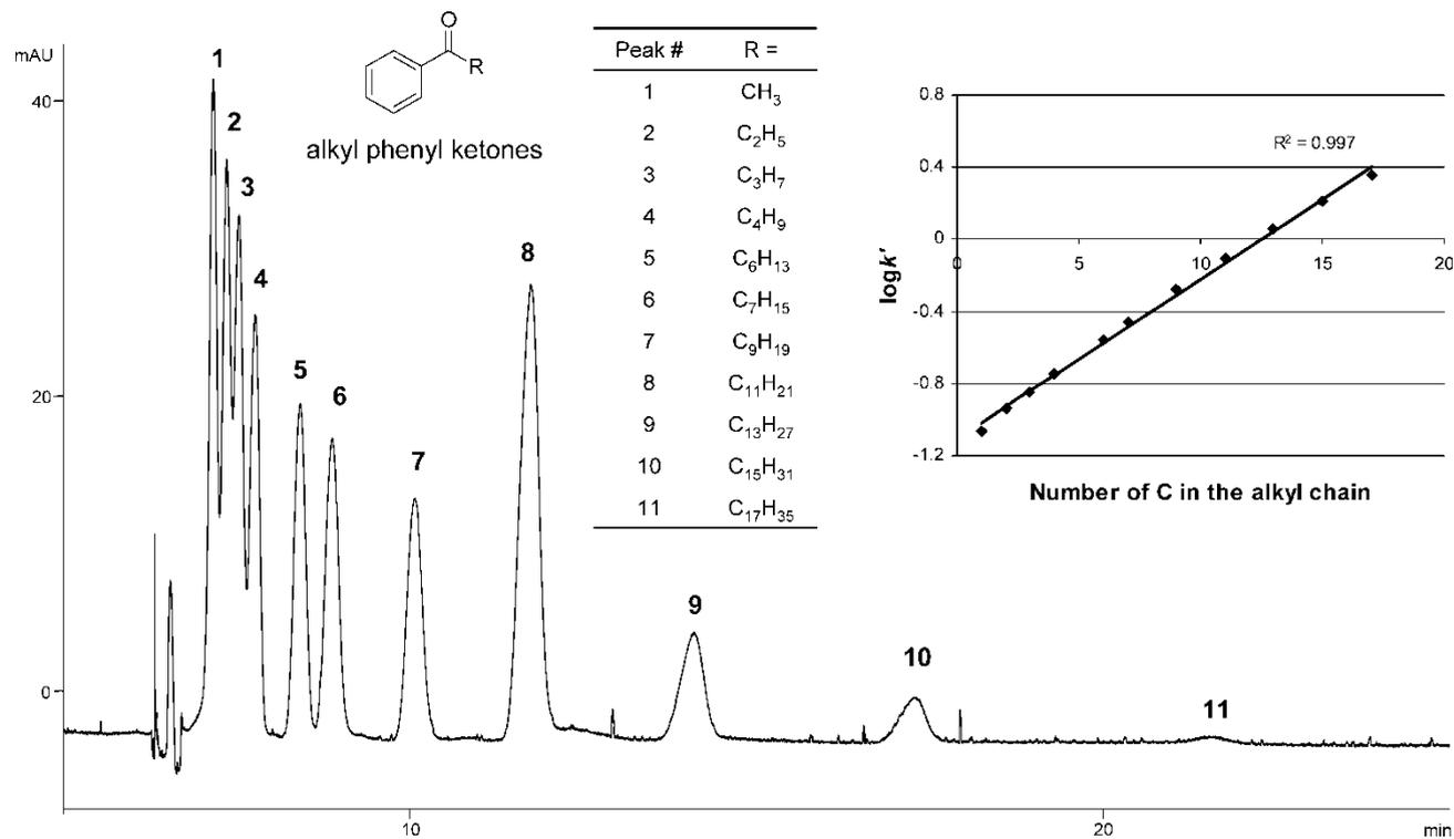
**Figure 3.** Electropherogram of CEC-UV separation of a test mixture of 11 alkyl phenyl ketones using the PSG column. The peak identification is listed in the inset table. Conditions are same as Figure 2.
